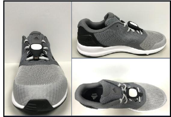
Figure 6. Sensor placement on top of the shoes
