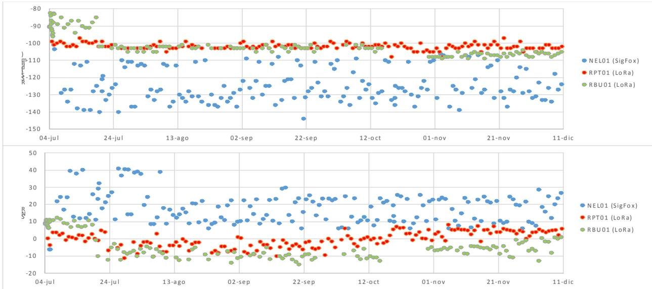
Fig 2. RSSI (above) and SNR (below) of LoRa and SigFox sensors in Puente Princesa
