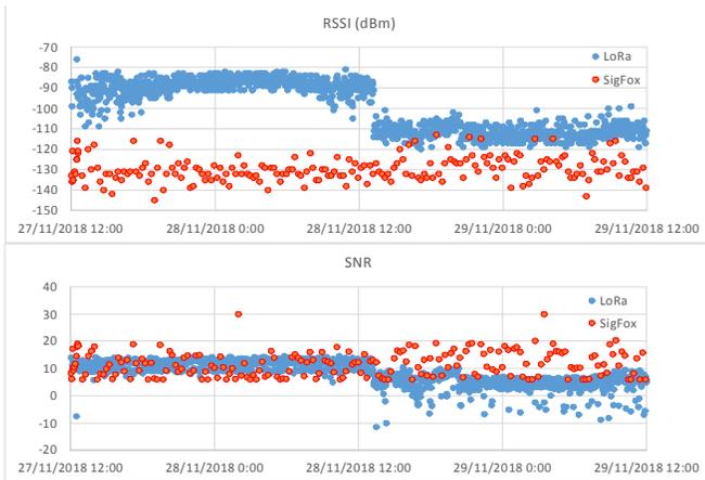
Fig 3. RSSI and SNR of LoRa and SigFox sensors in of testing deployment
