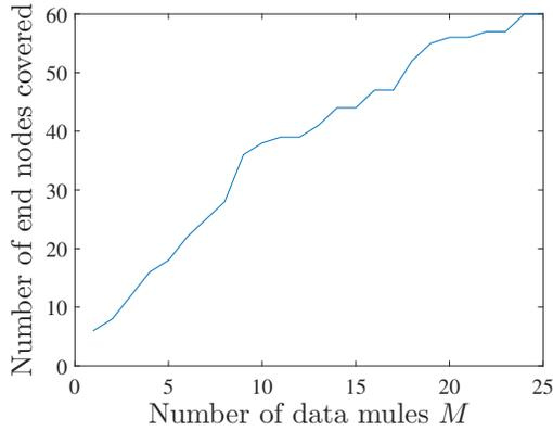
Fig. 8. Number of end nodes covered (out of a total 100) as a function of  $\mathcal{M}$  when  $t_s = 30s$ ,  $T_s = 180s$ ,  $t_a = 10$  ms,  $T_a = 1$  s, LOS range = 400m and overall data rate = 1 kbps.
