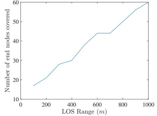
Fig. 10. Number of end nodes covered (out of a total 100) as a function of LOS range when  $\mathcal{M} = 25$ ,  $t_s = 30s$ ,  $T_s = 180s$ ,  $t_a = 10$  ms,  $T_a = 1$  s, and overall data rate = 1 kbps.
