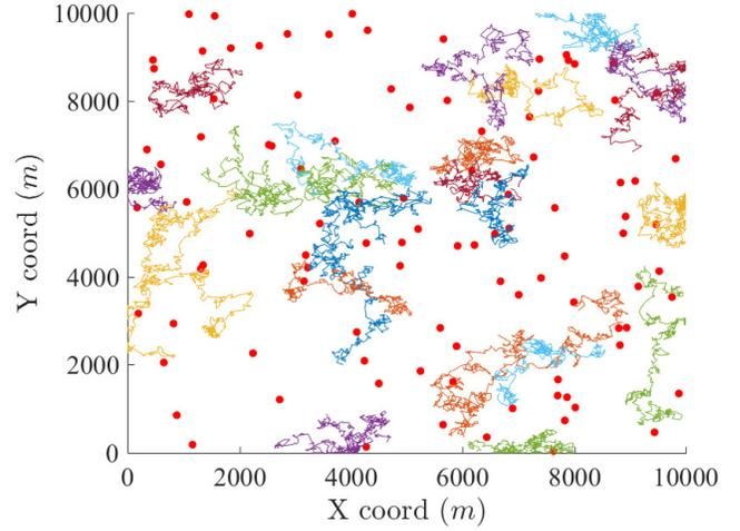
Fig. 6. Sample trajectories of data mules around the  $x - y$  grid. The red dots show locations of end nodes ( $\mathcal{N} = 100$ ) while the colored traces are the trajectories of data mules ( $\mathcal{M} = 25$ ).
