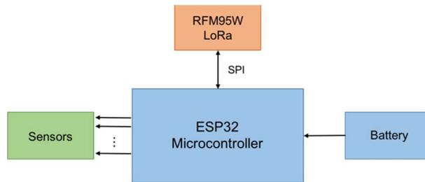
Fig. 3. Sensor node block diagram
