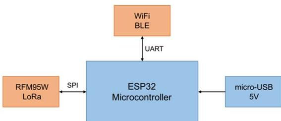
Fig. 2. Broke node block diagram
