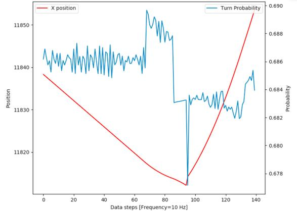
Fig. 4. Probability of right turn vs the X position of the vehicle
