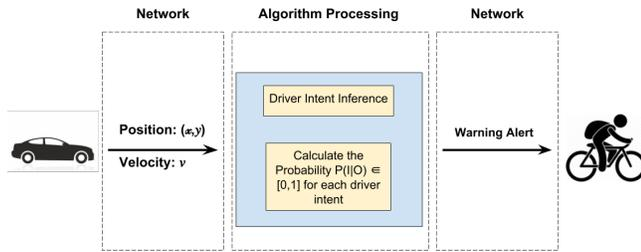
Fig. 1. Alert system's diagram: input from vehicle and output warning to cyclist.
