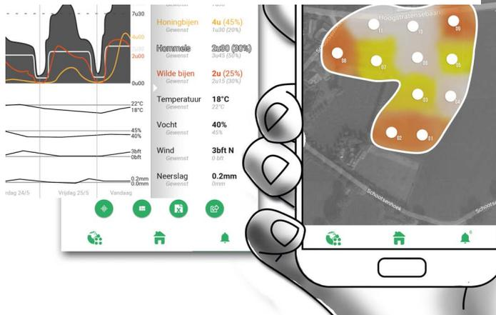
Fig. 3. The app is designed to provide users with the right information and feedback to take well-founded measures and to optimize the pollination situation on their field. For this the growers get a mapped view of the pollination factors on their field, daily advice on the basis of their personal data profile and a representation of the raw data to interpret themselves.
