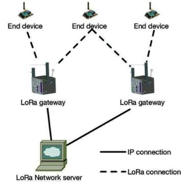
Fig. 1. LoRaWAN Network Architecture
