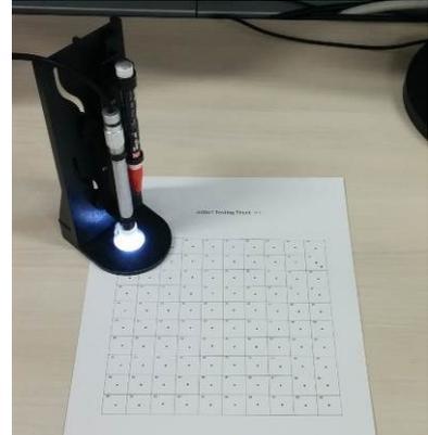
Fig. 6. Experimental setup to test accuracy of dot tagging and identification.
