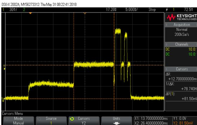
Fig. 7. Power measurement during data transmission
