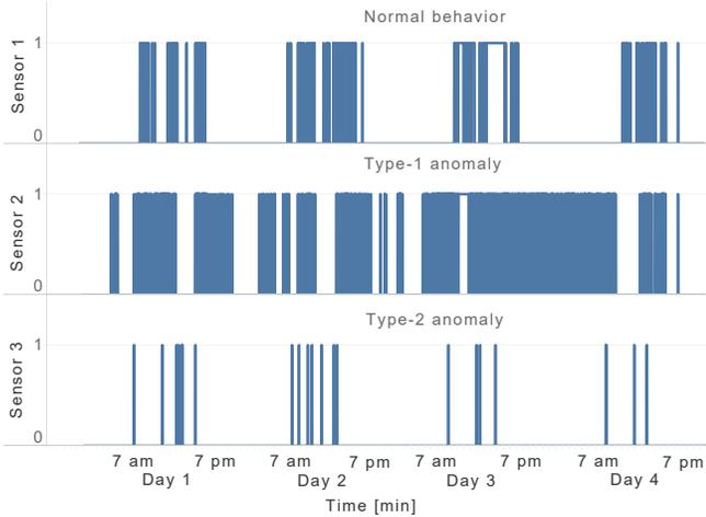
Fig. 1: Occupancy sensor data from three PIR sensors over one week.
