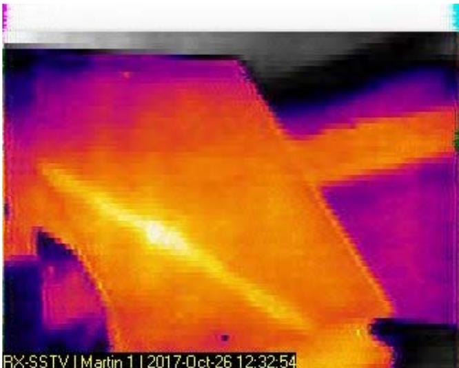
Figure VI Infrared Image of the PV panel on the AWQMS
