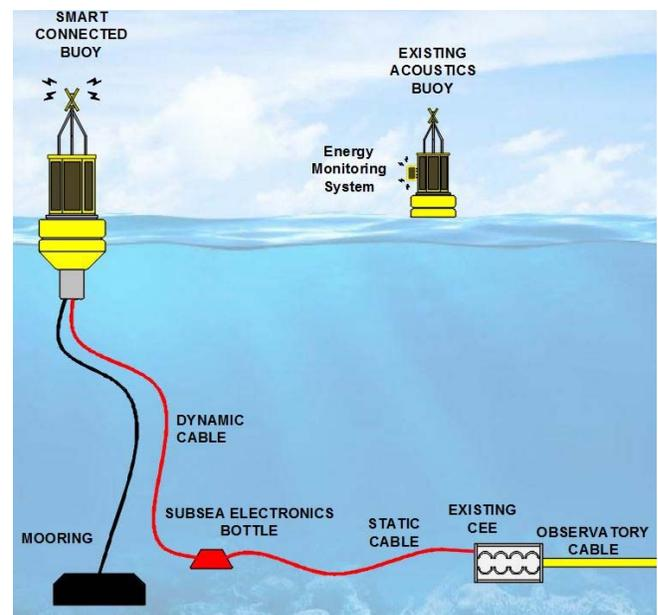
Figure I Energy Monitoring System deployed at Spiddal subsea observatory
