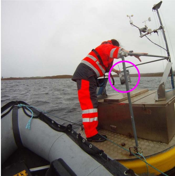
Figure V Energy Monitoring System being mounted on the AWQMS
