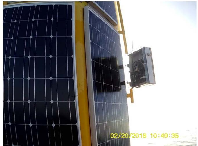
Figure II Energy Monitoring System clamped to handrail on Acoustic Buoy
