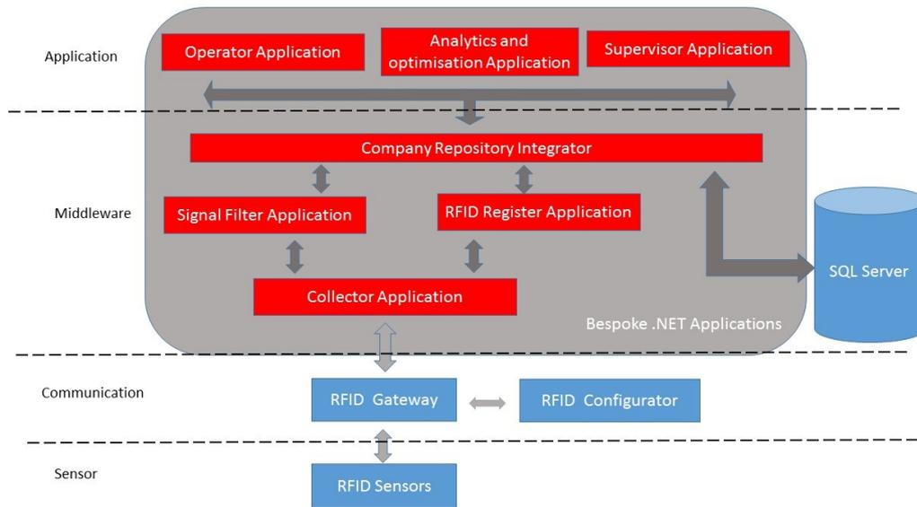
Fig. 2. Architecture for smart shelving
