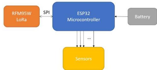
Fig. 2. Sensor node block diagram
