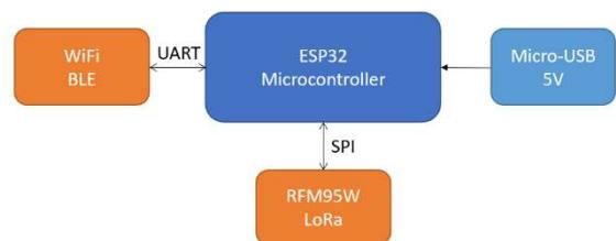
Fig. 4. Gateway block diagram
