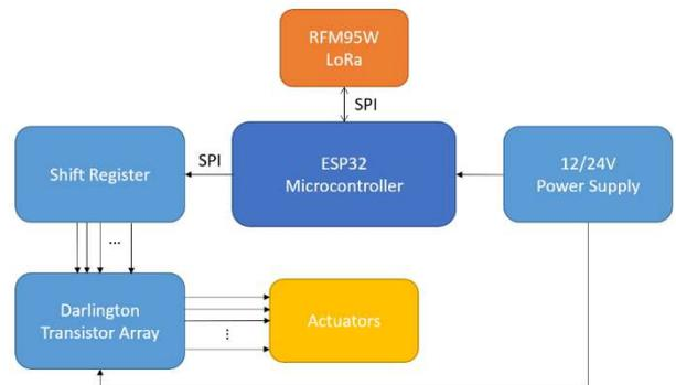
Fig. 3. Actuator node block diagram
