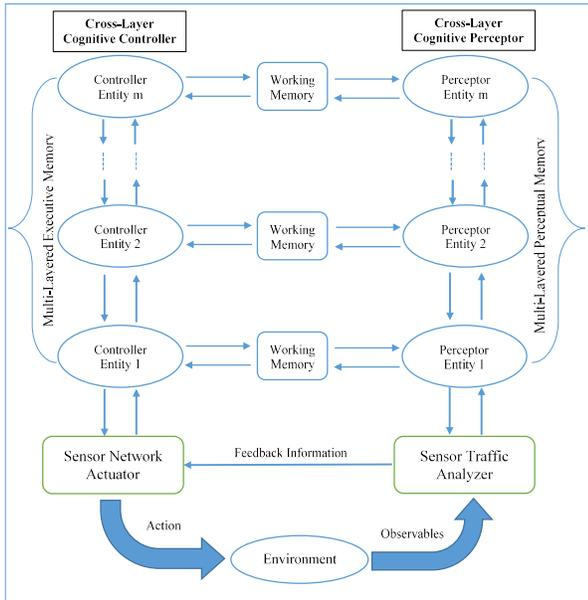
Fig. 1: Functional Block Diagram of the Cognitive IoT gateway as a Cognitive Dynamic System.
