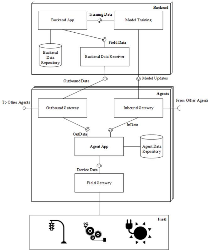
Fig. 1. Component view of the architecture
