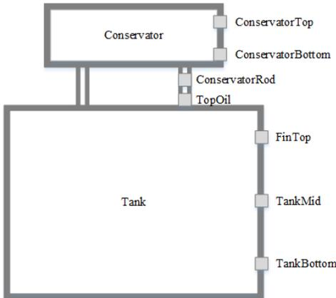
Fig. 2. Distribution transformer with placement of sensors
