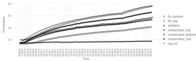
Fig. 5. Temperature modeling under normal operating conditions
